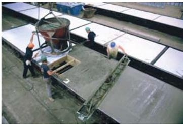
*Patented Superior Walls foundations are precision manufactured in factory-controlled conditions, then installed onsite in just hours.*
